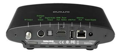
Plug in the Ethernet cable that is used to feed TV service into the Ethernet port on the STB.
